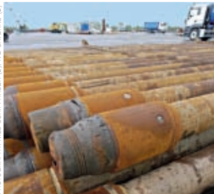
The caverns are created using drill strings of pipes bolted together.
